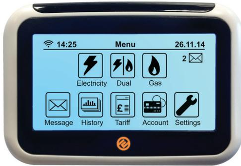
Your in-home display has a touch screen and gives you quick access to the status of your electricity and gas meter balance. It should be plugged into the mains at all times.
